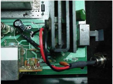
On the bottom of the board jumper the two negative leads together. Solder one end of the ceramic capacitor to the two negative leads you just jumpered.
