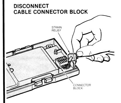
**1** Lift Cable Strain Relief UP and out of the housing.
