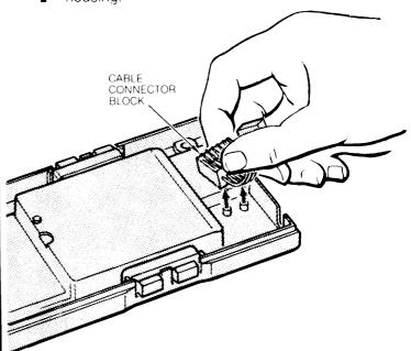
**2** Pry up Cable Connector Block from the housing.
