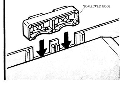
Before you replace the top make sure the Circuit Matrix and the Number Keypad are securely in place so that the top and bottom holes fit over the small brown posts.
