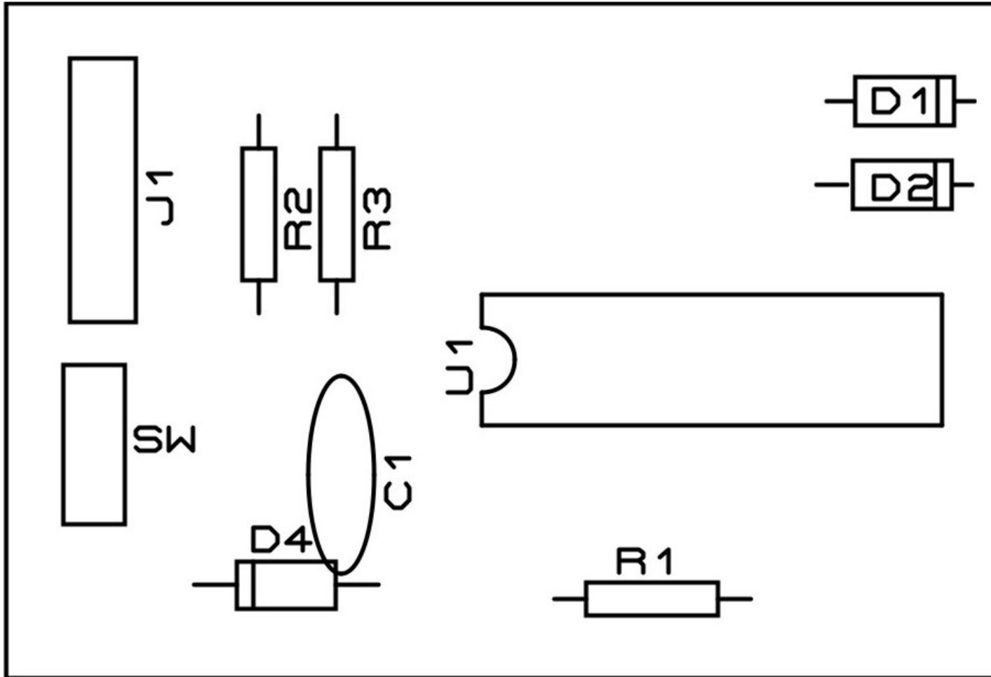
In the picture above we have the arrangement of the parts on the board. Note that the diodes and the IC has the right position to be assembled. The diodes have a ring close one of the terminals and IC has a semi-circle on one side.
