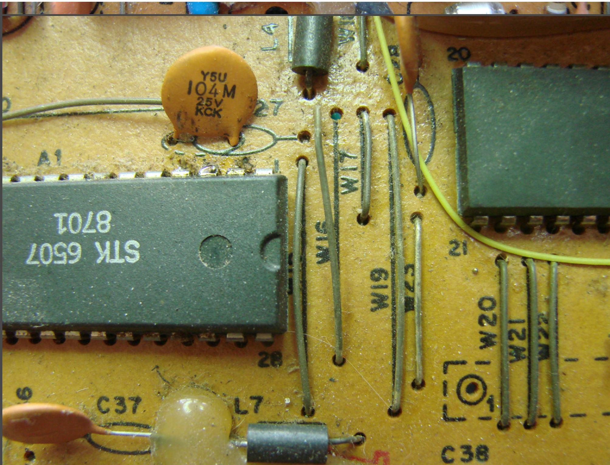
As I said before, the pictures above are from a Polyvox Atari. If you are doing this mod on another Atari or clone, follow the PCB track that goes from the CPU pin 3 to TIA pin 3. In the middle there is the 4k7 resistor, you must remove it, after that cut the track at any point with a sharp knife. Measure the track continuity with a multimeter after the cut.
