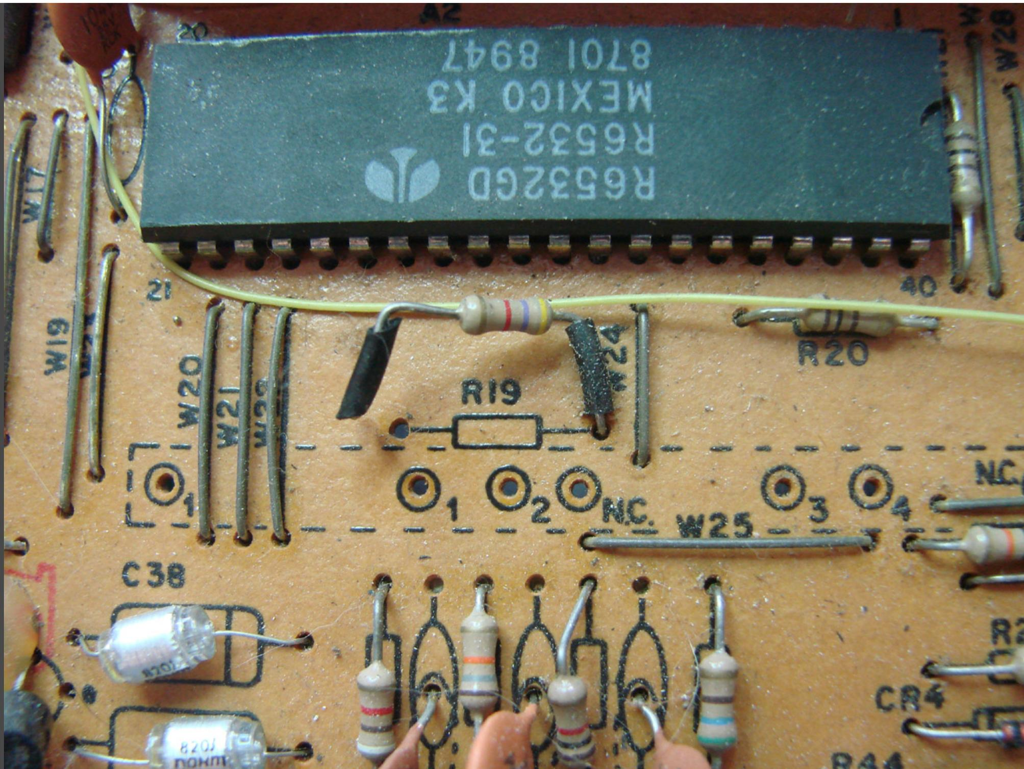
To break the connection between the pins, we will remove the jumper W16 at the right side of 6507.
