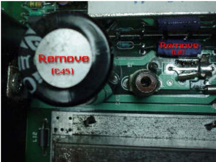
Next, install the 47uf electrolytic capacitor in C45 where you removed the other capacitor. Make sure to note polarity.
