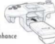
Note: When inserted into Expansion Slot 1 of the Dreamcast controller, the Vibration Pack connects, but does not lock. If the controller is jarred, the Vibration Pack may fall out during game play or otherwise inhibit game operation.
