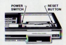
When returning to regular TV programming, slide the POWER SWITCH on the CONSOLE unit to "OFF". Slide the switch on the ANTENNA SWITCH BOX back to "TV" position.
