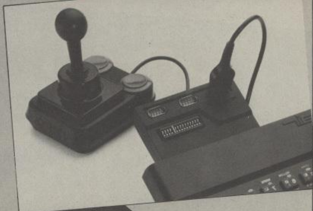
Above: a conventional joystick with upright stick and two fire buttons on the base. This one is Kempston's Competition Pro.
