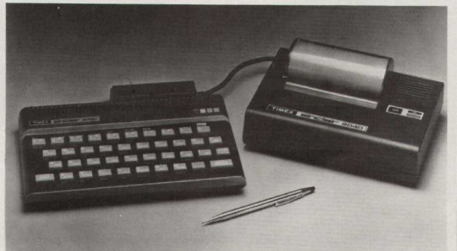
A dot matrix printer can be used with Timex' computers.
